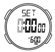
Press "D" to increase the hour, press "C" to decrease the hour, press and hold to adjust at high speed;
