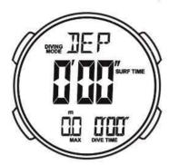
2. The diving time on, when the diving depth more than 1.2m or 4Ft (" WODE " flashing);
