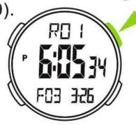
In the F01~99 state, press "C" to browse the selection in the following sequence: Dive start time, date → Max. diving depth, temperature, diving time, surface time → the average diving depth, diving time, surface time.
