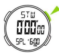
To display the SPL1 time by pressing "D" again (Auto running after 2 seconds);
