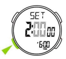
Press "D" to increase the number, press "C" to decrease the number, press and hold to adjust at high speed;
