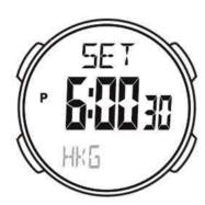
Press "C" or "D" to select the city code, press and hold to adjust at high speed;
