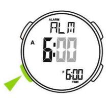
4. Press "D" to increase the minutes, Press "C" to decrease the minutes, press and hold to adjust at high speed;
