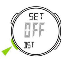
4. Press "C" or "D" to ON/OFF the Daylight Saving Time.
