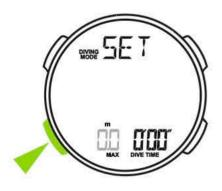
Press "D" to increase the number, press "C" to decrease the number, press and hold to adjust at high speed;
