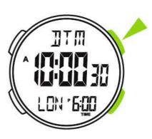
In the world time mode, press and hold "A" to ON/OFF the Daylight Saving Time.
