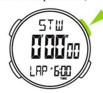
Display the LAP1 time by pressing "D" again (Auto running after 2 seconds);
